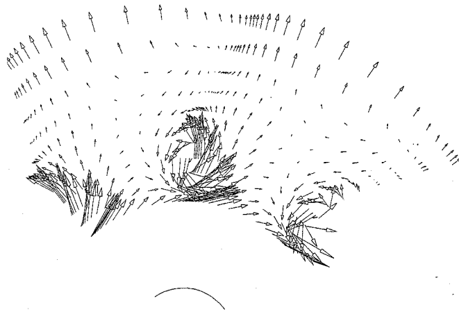
Fig. 9 Velocity vectors behind the rear blade.
